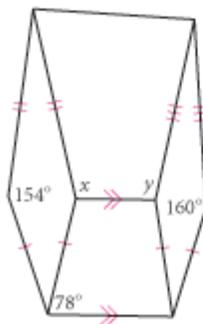
18. What is the measure of each angle in the isosceles trapezoid face of a voussoir in this 15-stone arch?
